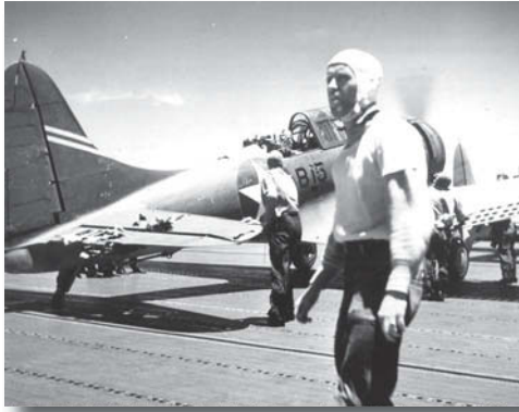
A Douglas SBD-3 "Dauntless" scout bomber, of USS Enterprise's Bombing Squadron Six (VB-6), on the USS Yorktown (CV-5) during the Battle of Midway. The newly installed electrical arming system resulted in the premature release of bombs. (Photo courtesy of US Navy Historical Center)
